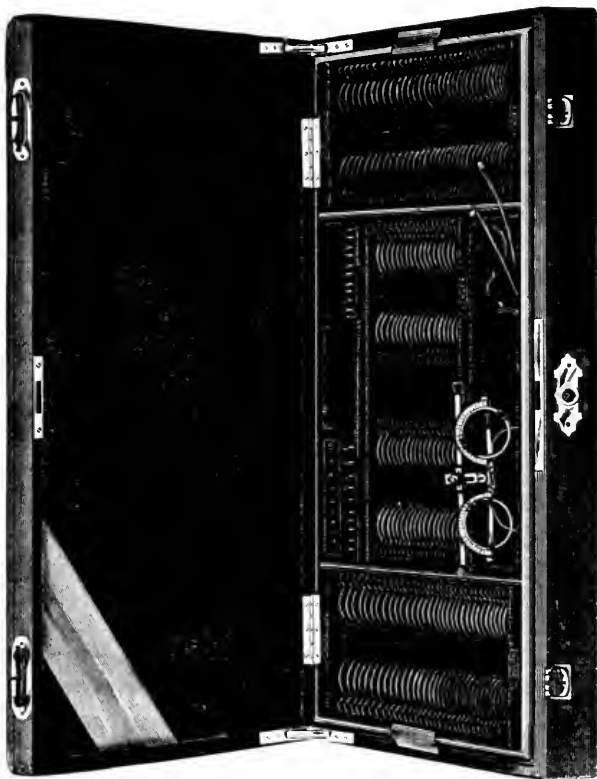
Trial Case Containing Various Lenses Needed for Testing the Refraction of the Eyes.
